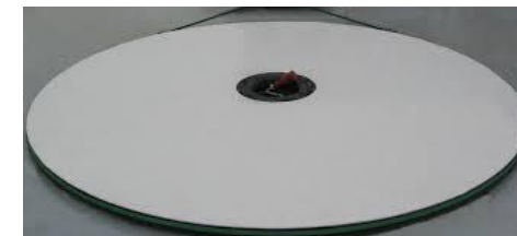
Rotating Table: To rotate EUT for testing
