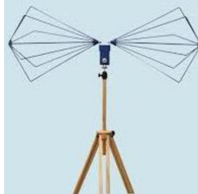
Biconical Antenna: 30 to 300 MHz
